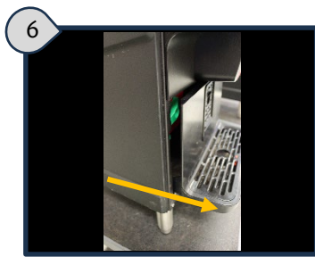
Remove and empty the drip tray.
