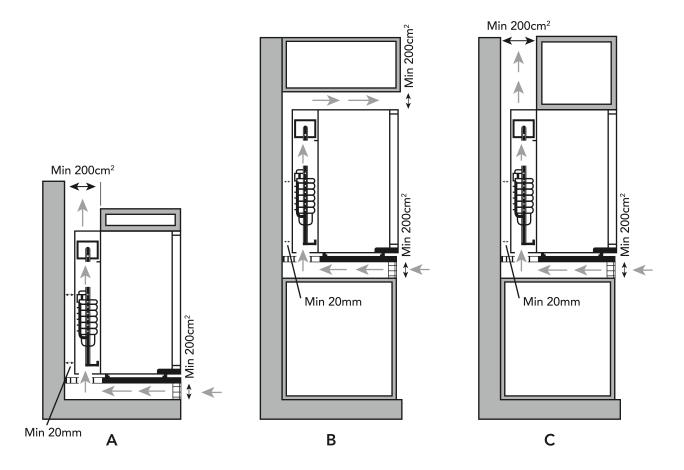
The premise is to create a chimney effect in the back of unit. Cold air enters the furniture at the base, passes through the cooling system and the warm air rises and escapes.
