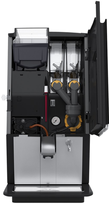
Esprecious 12 (shown open): Grinder (1), Whole bean hopper (1); holds up to 3.0 lbs., Soluble canisters (2); holds up to 2.0 lbs. each. Esprecious 22: Grinder (2), Whole bean hopper (2); holds up to 1.5 lbs. each. Soluble canisters (2); holds up to 2.0 lbs. each.
